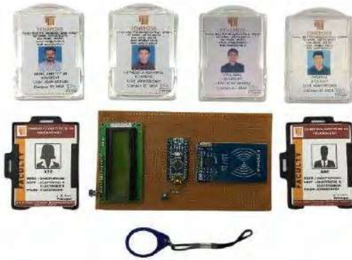
Fig. 3: Real project kit and its RFID cards, tag
